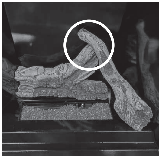
Figure 75: Using a 5/16 drill bit, drill a hole 1in deep in the rear log as shown above. Insert the log pin that was supplied with the unit into the hole.
