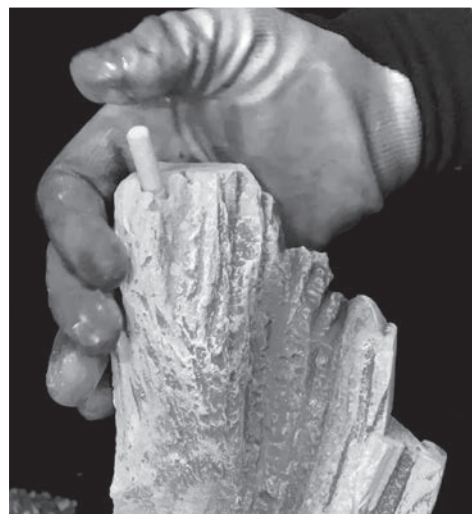
Figure 75: Using a 5/16 drill bit, drill a hole 1in deep in the rear log as shown above. Insert the log pin that was supplied with the unit into the hole.
