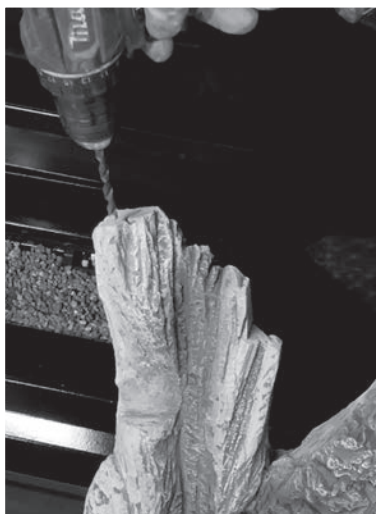
Figure 75: Using a 5/16 drill bit, drill a hole 1in deep in the rear log as shown above. Insert the log pin that was supplied with the unit into the hole.
