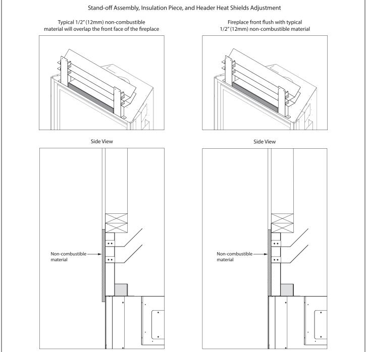
FIGURE 3.1 Stand-off Assembly, Header Heat Shields, and Insulation Piece Adjustment
