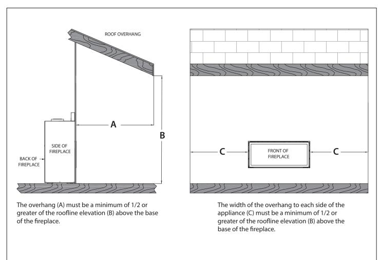
EXAMPLE: If roofline (B) is 10' above the base of fireplace, the overhang (A) must be 5' or greater. The width of the overhang to EACH side of the fireplace (C) must be 5' or greater.
