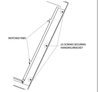
FIGURE 4.9 Screw Location on Hanging Bracket
