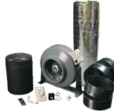
An optional 635 cfm external blower can be used to circulate the heat from the fireplace in any direction. The kit includes a 5 ft. length of acoustic ducting, a variable speed control, a mounting bracket and a back draft damper. Can be installed on the left side only.
