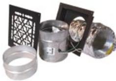
The Heat Dump Kit uses a 180 cfm fan to direct a moderate amount of warm air from the fireplace to another room. It has a maximum run of 8 ft. and is most often used to provide supplemental heating to a basement room when the fireplace is on the main floor.
